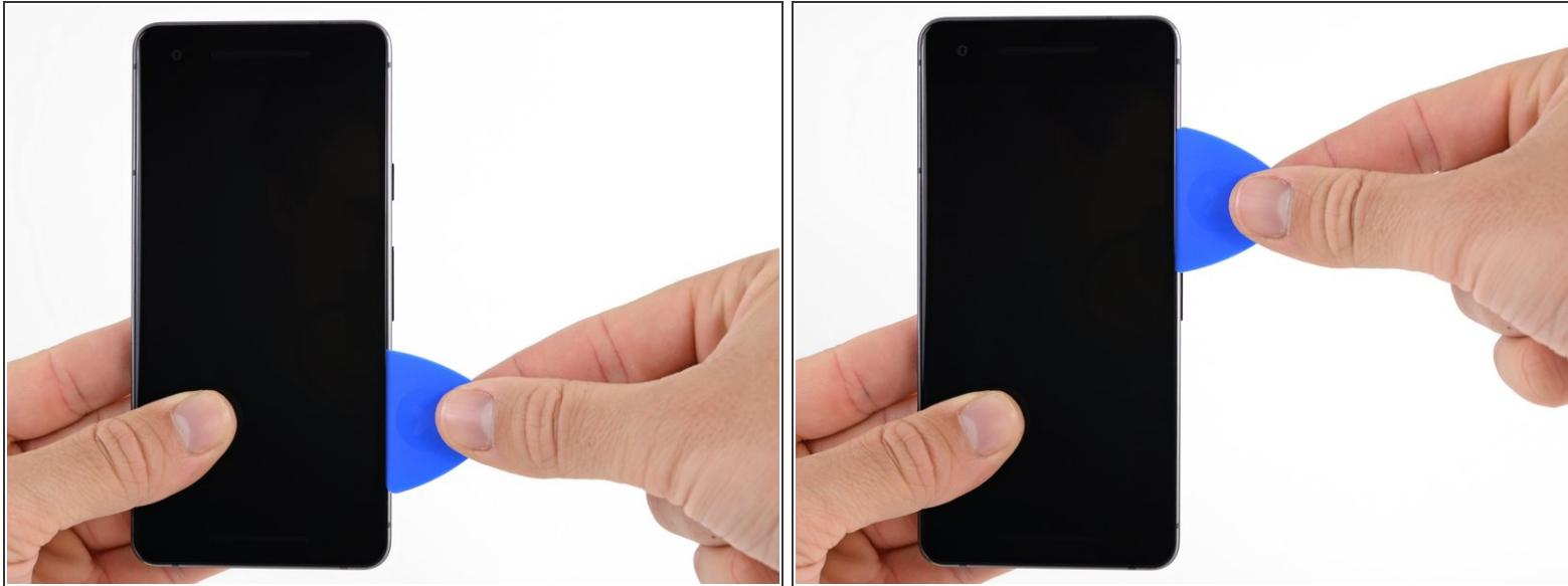
*(i)* In the following steps, use the flat of the opening pick, rather than a corner, to cut here. This will help prevent inserting the pick too deeply.
